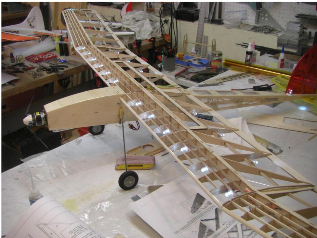
FORWARD LEDs MOUNTED UNDER CENTER TURBULATOR, NOTE THE FIRST TURBULATOR IS REMOVED FROM THE BAY. USE MAGNET WIRE FOR CONNECTIONS
